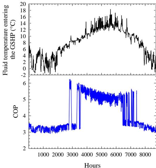
Figure 9: Hourly values of fluid temperature entering the GSHP and corresponding COP.
