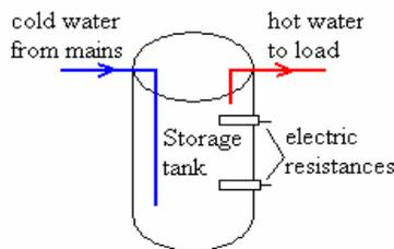
Figure 2: Electric water heating (Alternative 1)
