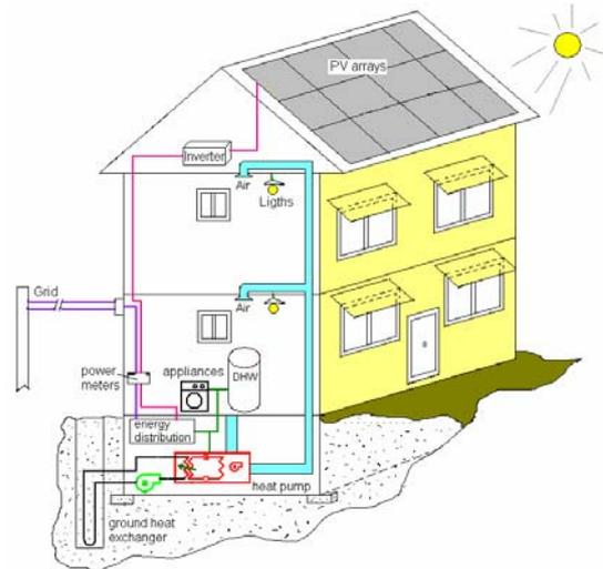
Figure 1: Schematic representation of the ZNEH studied here
