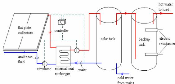
Figure 4: Solar domestic water heating system (Alternative 3)
