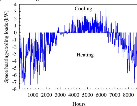
Figure 8: Hourly space heating and cooling loads
