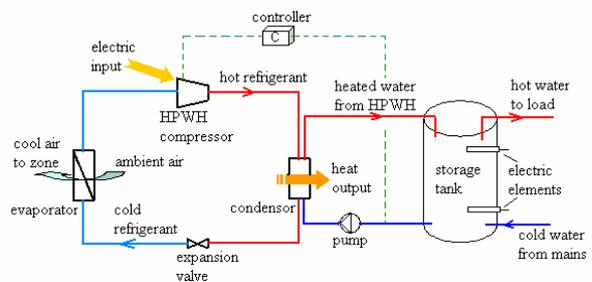
Figure 5: Heat pump water heater system (Alternative 4)
