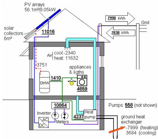
Figure 11: Energy flow of the ZNEH with solar collectors
