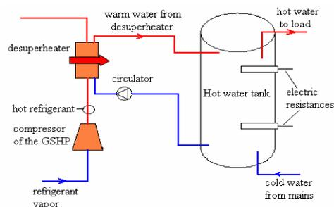
Figure 3: Domestic hot water heating using a desuperheater (Alternative 2)
