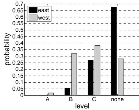
Figure 7 Probability of the thermal comfort (ATG) of cross night ventilation in a west and east office.
