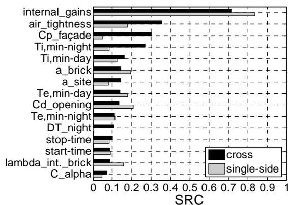
Figure 8 Most influential input parameters of cross and single-sided night ventilation compared
