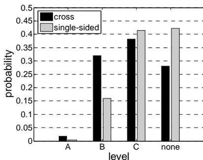
Figure 6 Distribution of thermal comfort of single-sided and cross night ventilation in a west office.
