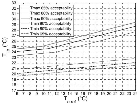
Figure 1: ATG-method in naturally ventilated buildings: limiting internal temperatures
