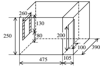
Figure 2 Two-zone model of single-sided natural night ventilation
