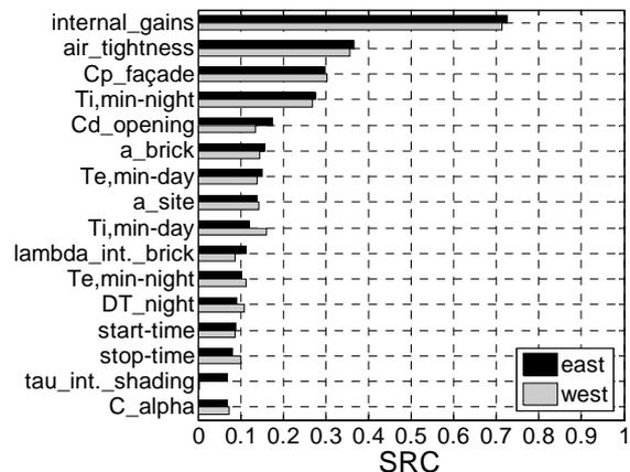
Figure 9 Most influential input parameters of cross night ventilation in a west and east office compared
