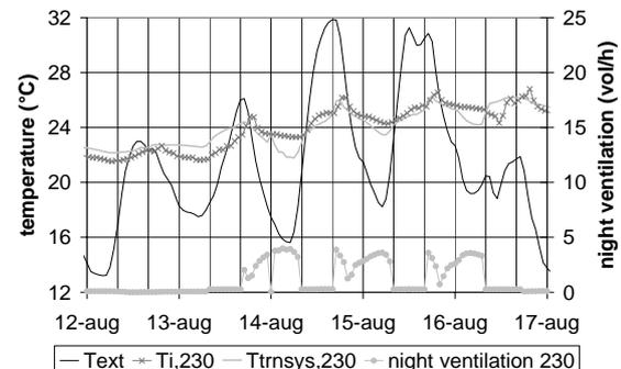
Figure 5 Comparison of simulated and measured operative internal temperature in a west office of Probe-building.
