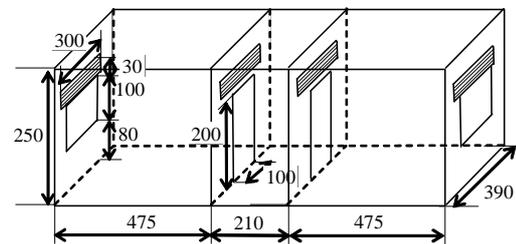
Figure 3 Three-zone model of cross natural night ventilation
