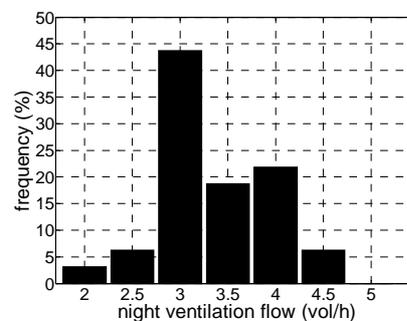
Figure 4 Distribution of average single-sided night ventilation rate in a west office of Probe-building
