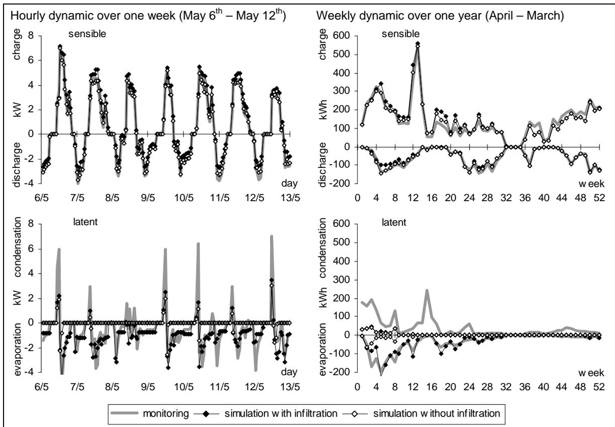
Figure 7 : Geoser, comparison of monitoring and numerical simulation.
