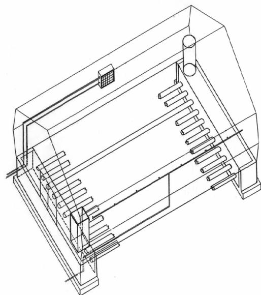
Figure 5 : Geosier greenhouse with buried pipe system.
