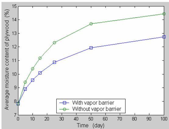
Figure 6 Average moisture content of sheathings with and without vapor barrier
