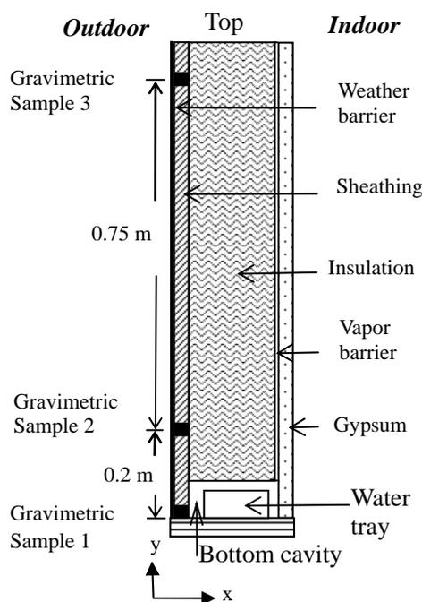
Figure 1 Sketch of experimental setup, a water tray is put at the bottom of stud cavity
