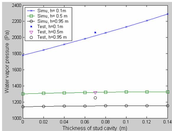
Figure 3 Comparison of Vapor pressure in study cavity by simulation and test
