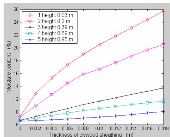
Figure 5 Moisture distribution through the thickness of plywood sheathing at different height
