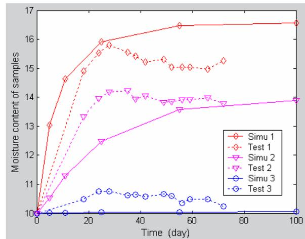
Figure 4 Comparison of Moisture contents of sheathing panel from gravimetry and simulation
