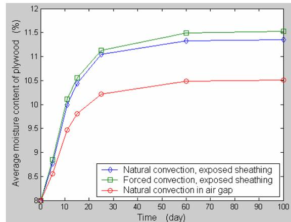
Figure 7 Average moisture content of plywood sheathing under various convective conditions
