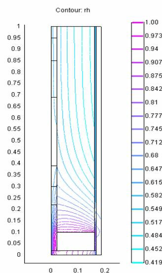
Figure 2 Contour of relative humidity in envelope
