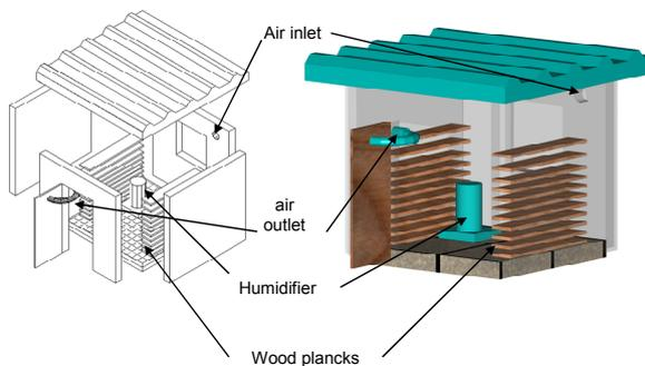
Figure 3 : LGI test cell for buffer model validation
