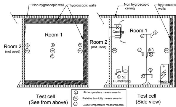
Figure 4 : Test cell called “STAttron” (side view and above)
