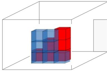
Figure 5 Dynamically varying transparency to eliminate of view obstruction.
