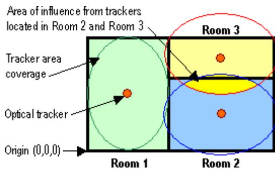
Figure 3 A sample three-room AR hardware preparation – plan view.
