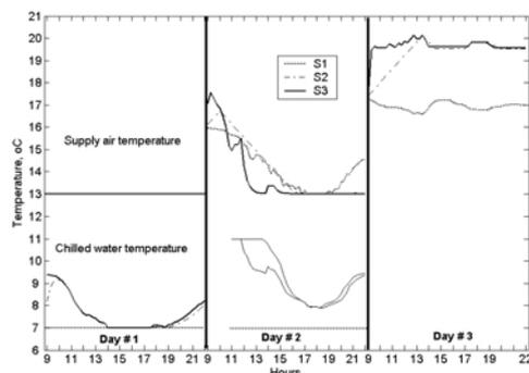
Figure 8 Supply air and chilled water temperature set points of AHU-4 for three days
