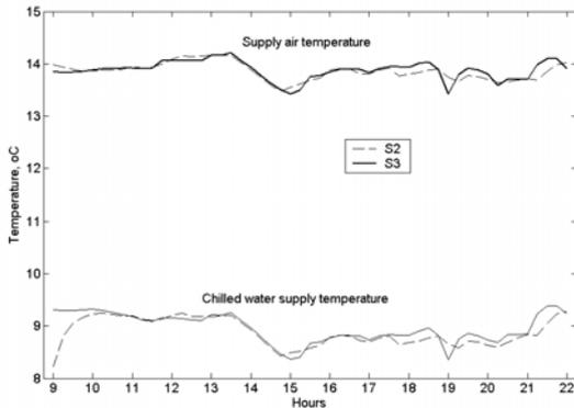
Figure 4 Supply air and chilled water temperature set points in AHU-6 for summer day
