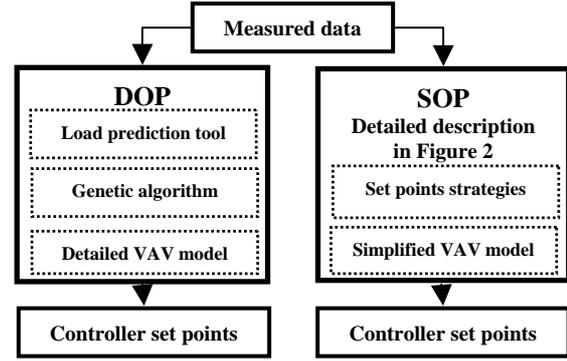
Figure 1 Schematics of the detailed and simplified optimization processes (DOP and SOP)
