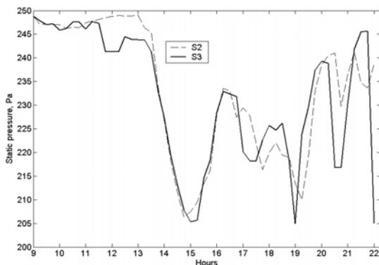
Figure 5 Duct static pressure set point in AHU-6 for summer day
