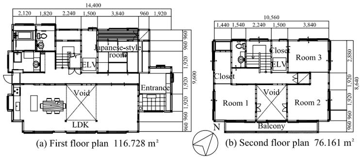
Figure 8 The first and second floor plans
