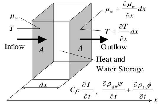
Figure 1 Conductive heat and moisture transfer
