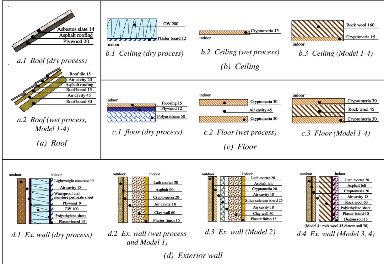
Figure 9 Wall assemblies of building model
