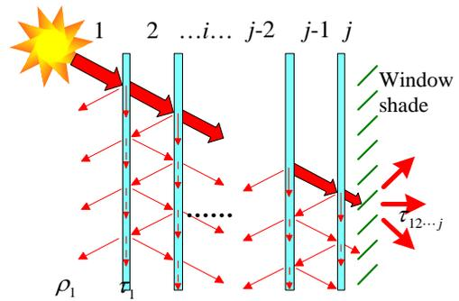
Figure 4 Multi-layer window model
