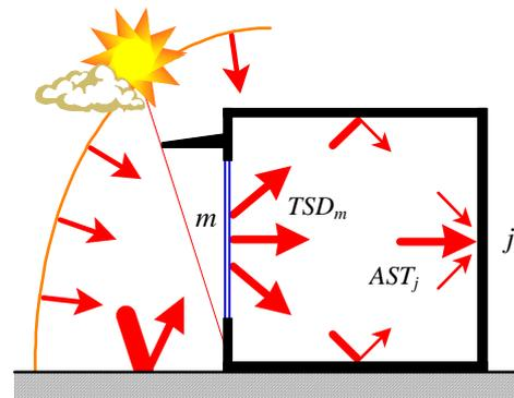
Figure 6 Multiplex reflection of transmitted sky diffuse solar radiation
