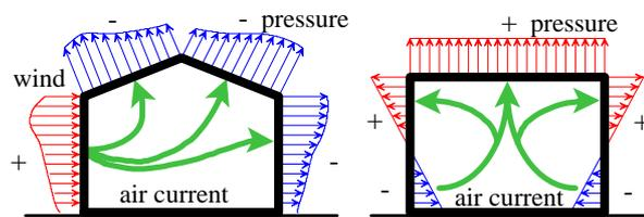
(a) Wind forced ventilation (b) Buoyant ventilation
