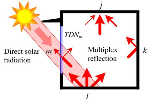
Figure 5 Multiplex reflection of transmitted direct solar radiation
