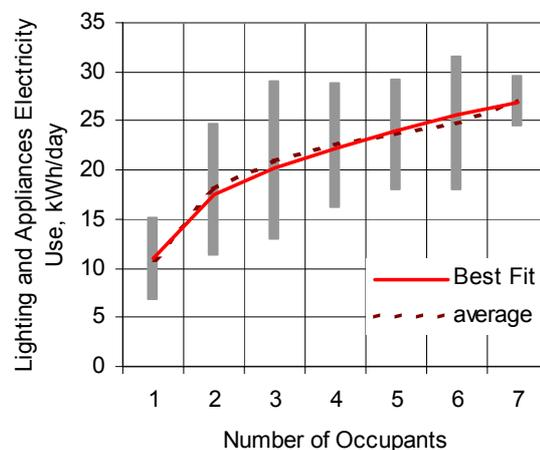
**Figure 2. Profile of base loads in single-family housing.**
