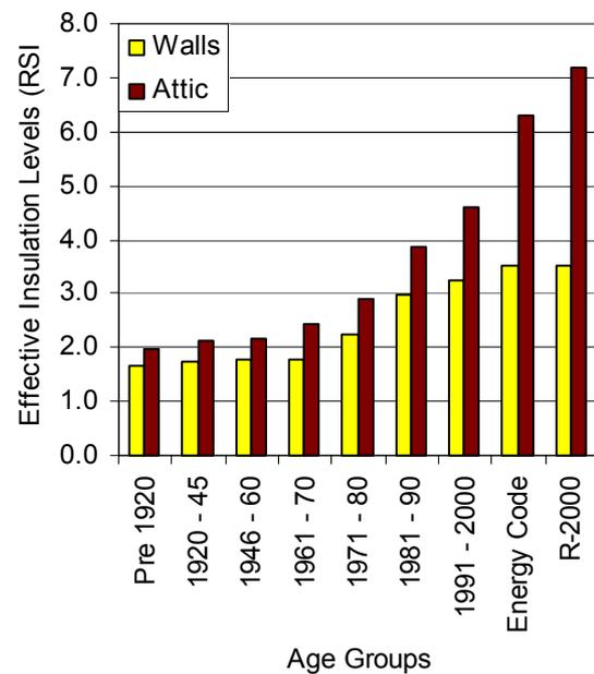
Figure 7. Improvements in envelope insulation.
