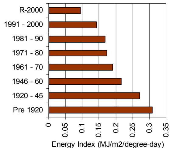
Figure 8. Energy use index for space heating and hot water use in Canadian housing.
