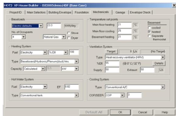
Figure 5. Data input for the mechanical systems.
