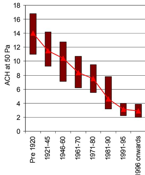
**Figure 1. Airtightness characteristics for the Quebec housing – bottom of the bar is at 25<sup>th</sup> and top is at 75<sup>th</sup> percentiles.**
