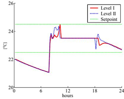
(c) Room air temperature profile (after HVAC's operation at each sampling time)
