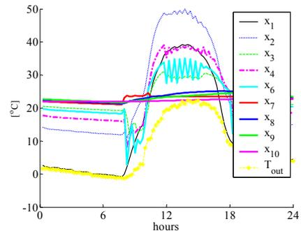
(a) State variable and outdoor air temperature (Level I control)
