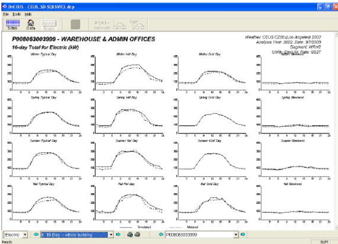
Figure 7 16-Day Whole Building Load Shape and Interval Metered Data
