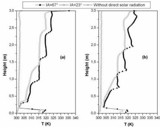
Figure 4 Temperature profiles inside the channel of the double-skin placed at 0.062m and 0.162m from the external glazing ((a) and (b) respectively).
