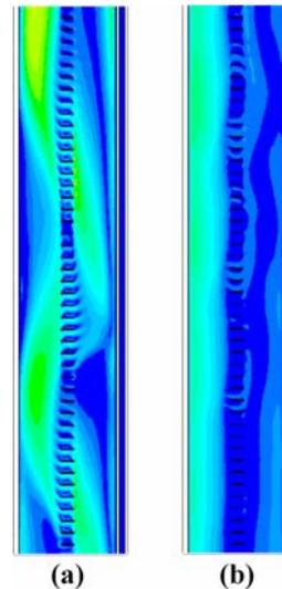
Figure 3 Iso-velocities inside the channel of the double-skin with and without direct solar radiation ((a) and (b) respectively).
