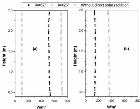
Figure 5 Radiation heat flux on the external surface and the transmitted solar radiation flux to the inside of the building ((a) and (b) respectively).
