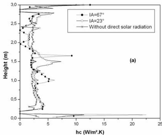
Figure 7a Convective heat transfer coefficient of the external glazing.
