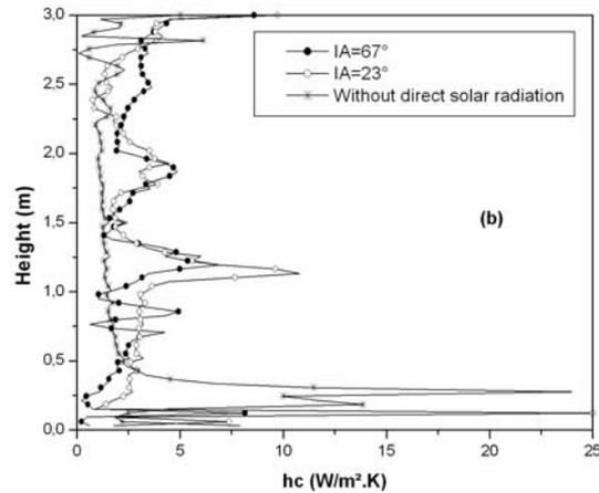
Figure 7b Convective heat transfer coefficient of the internal glazing.
