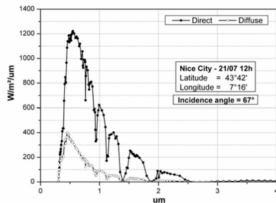
Figure 2 Spectral representation of the direct and diffuse solar radiation (south orientation).
