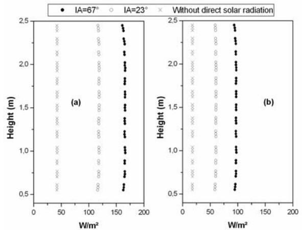
Figure 6 Reflected radiation flux on the external surface for the first band (0 – 0.78  $\mu\text{m}$ ) and the second one (0.78 – 2.7  $\mu\text{m}$ ) ((a) and (b) respectively).
