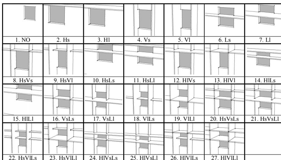
Figure 1 Different shading/lighting systems that were analyzed. H=horizontal louver, V=vertical louver, L=lightshelf; s=small=50 cm, l=large=100 cm
