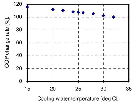
Figure 6. COP change by cooling water temperature
