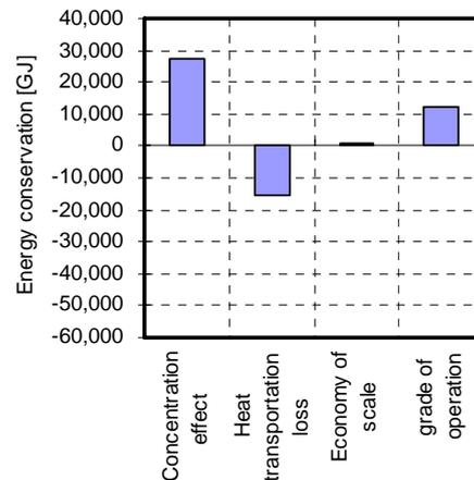
Figure 15. Effects of the factors on cooling.
