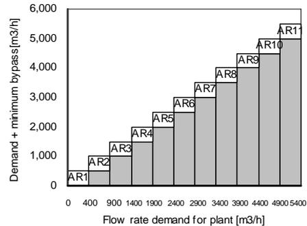
Figure 10. Chiller control sequence by flow rate
