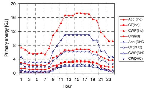
Figure 13 Hourly change of energy consumption of pumps and other machines.
