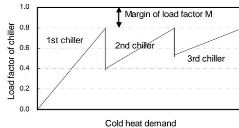
Figure 7. Margin of load factor
