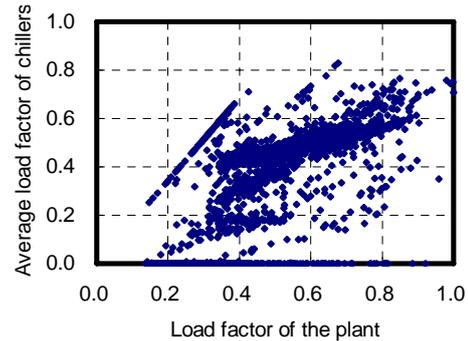
Figure 9. Multiple chiller sequence in individual plant
