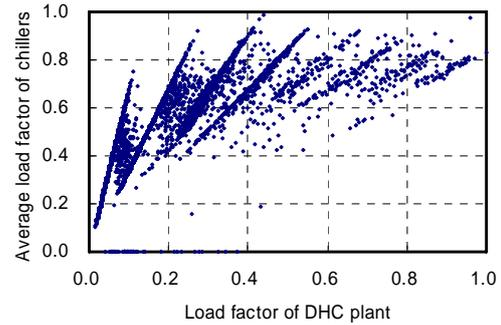
Figure 8. Multiple chiller sequence in DHC plant
