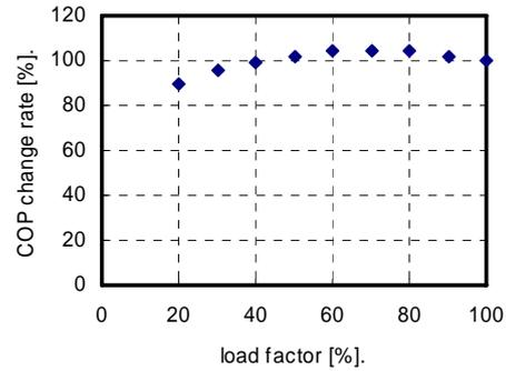
Figure 5. COP change by load factor
