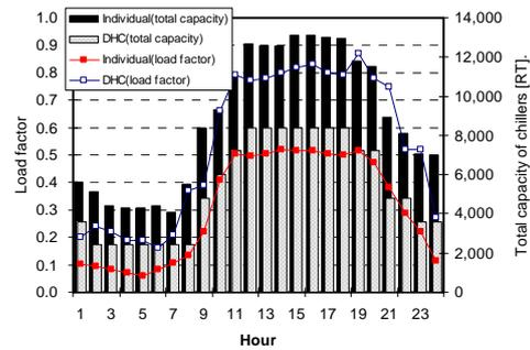
Figure 12 Hourly change of chiller sequence on 15<sup>th</sup> June.
