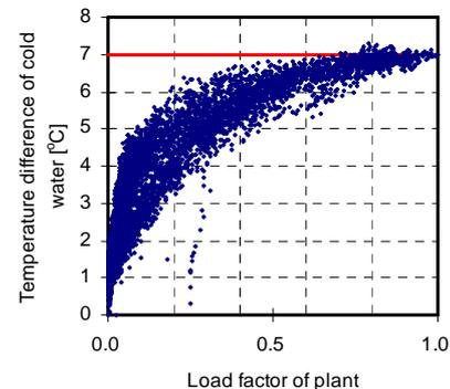
Figure 11. Relationships between cooling load and temperature difference in cold water in the A-Plant.
