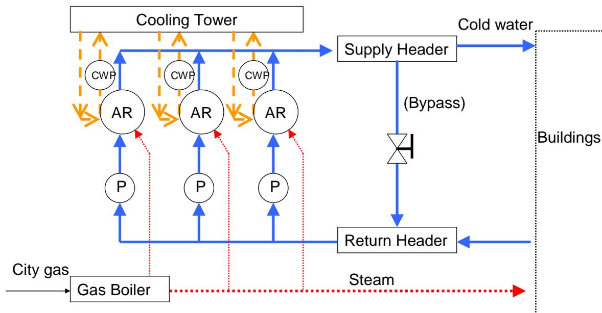
AR: absorption chiller, P: cold water pump, CWP: cooling water pump
