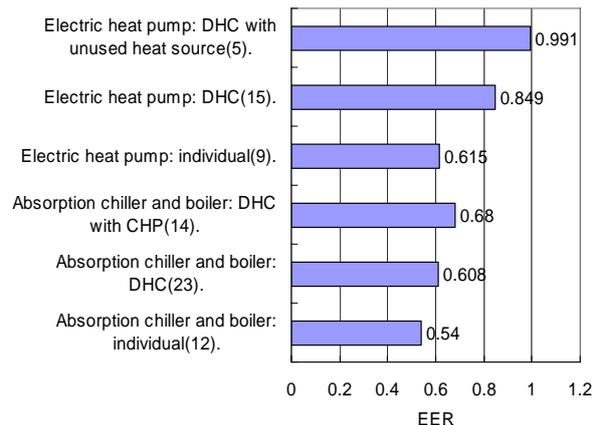
Figure 1. Average EER of DHC and individual system [( )= number of sample]
