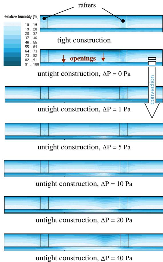
Figure 3 Relative humidity field in the slope roof construction – the case of air infiltration
