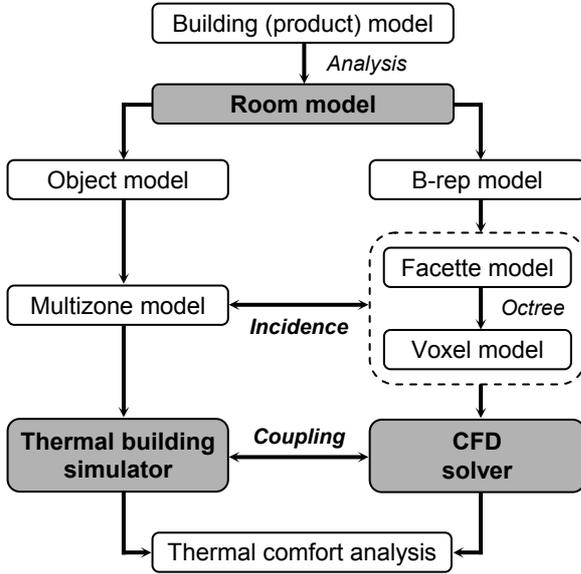
Figure 2: Sequence of operations within the discretization process
