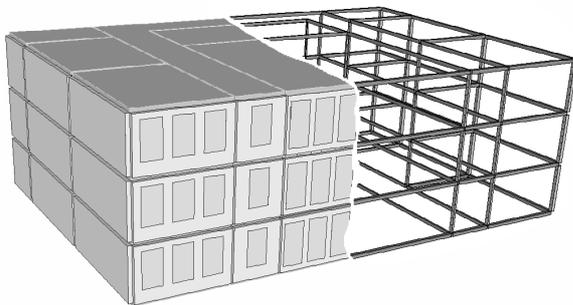
Figure 9: Decomposed model with difference and coupling objects, respectively
