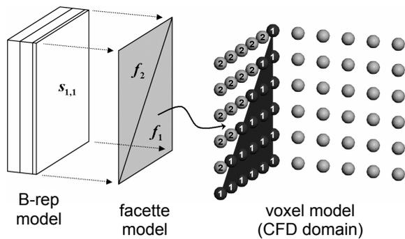
Figure 15: Link between B-rep model and voxel model (CFD domain)
