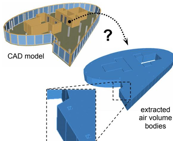
Figure 1: Single floor of multi-storey office building and corresponding set of (here) four air volumes
