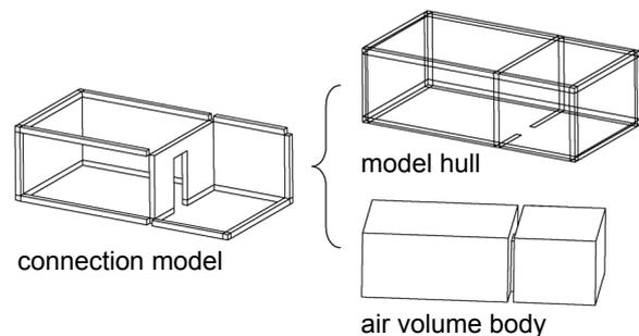
Figure 7: Air volume extraction of model with two rooms being connected by open door
