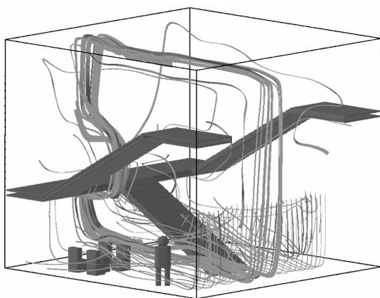
Figure 17: Natural convection in inner courtyard induced by boundary conditions computed by a thermal multizone simulation (streamlines are injected at horizontal plane at front facade)
