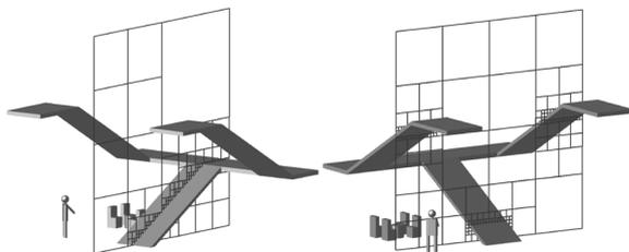
Figure 16: Vertical cut through octree discretization (quadtree representation, levels 0 to 6 displayed)
