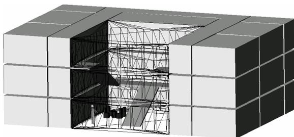
Figure 13: Facetted surface mesh of CFD domain with staircase and occupants
