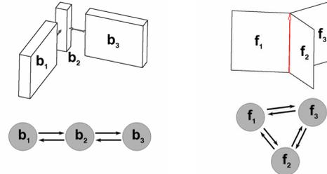
Figure 3: Structural component graph (left) and graph of room faces (right)
