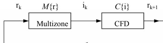
Figure 3 Schematic of the coupling procedure at the coupling iteration  $k$
