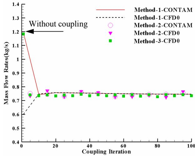
Figure 5 Airflow rate through Path B during the iteration with the three coupling methods in a 4-zone building model with cross ventilation
