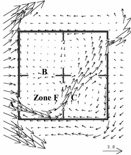
Figure 4 The experimental airflow pattern for the 4-zone building model with cross ventilation
