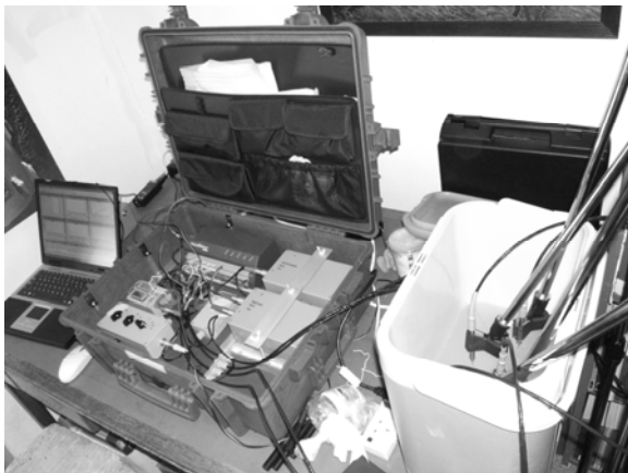
Figure 1: experimental thermal probe measurement kit (during calibration phase, measuring agar immobilised water)
