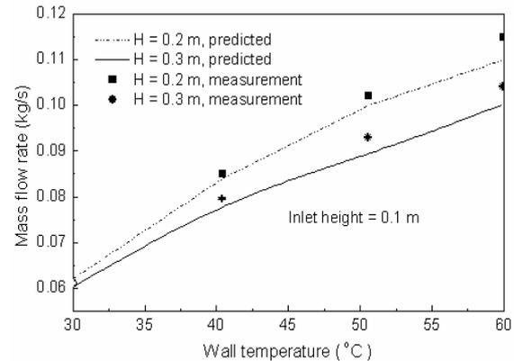
Figure 3. Comparison between the predicted results of mass flow rate and experimental data
