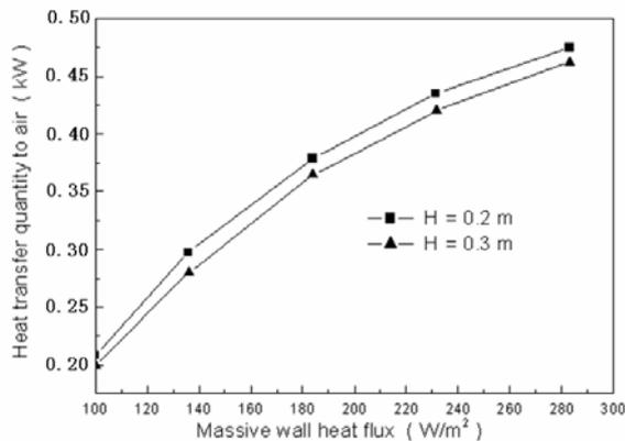
Figure 4. Quantity of heat transfer to air in channel
