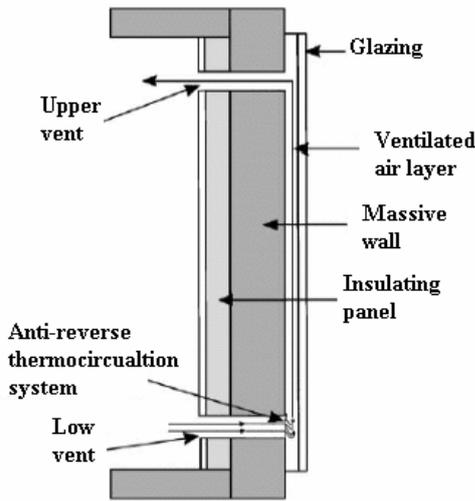
Figure 1. Schematic diagram of insulated Trombe wall
