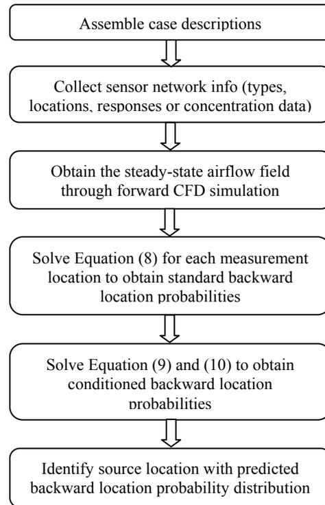
Figure 1 Flow chart of the CFD-based adjoint inverse modeling method for contaminant source location identification
