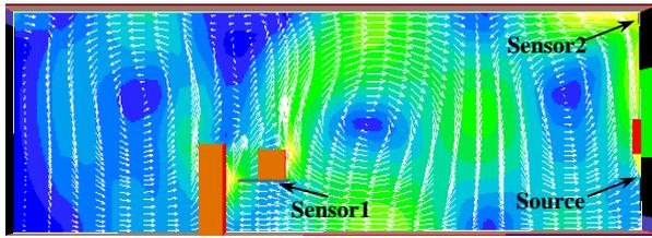
Figure 2 CFD office model and predicted airflow field
