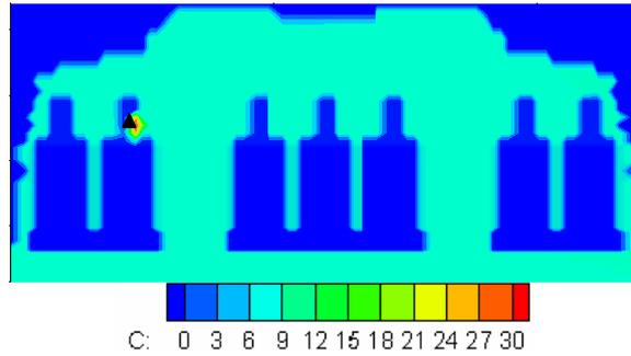
Figure 9 Predicted source location probabilities (%) by the joint probability method with two one-time-reading sensors for the cabin case
