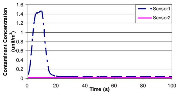
Figure 7 Predicted contaminant concentration variations at the two sensor locations during the first 100 seconds after the contaminant was released in the cabin
