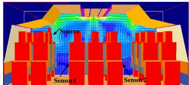
Figure 6 Geometry, configuration, predicted main airflow pattern, and source and sensor locations of the aircraft cabin model
