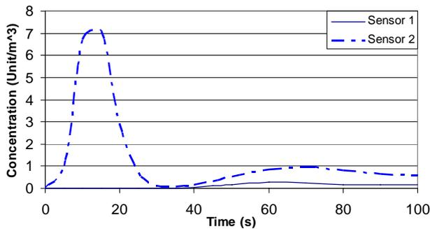
Figure 3 Predicted concentration temporal variations at the two sensor locations in the office
