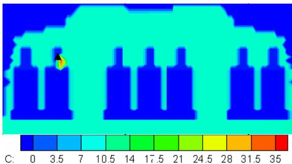
Figure 8 Predicted source location probabilities (%) by the joint probability method with one one-time-reading sensor (sensor 1) for the cabin case
