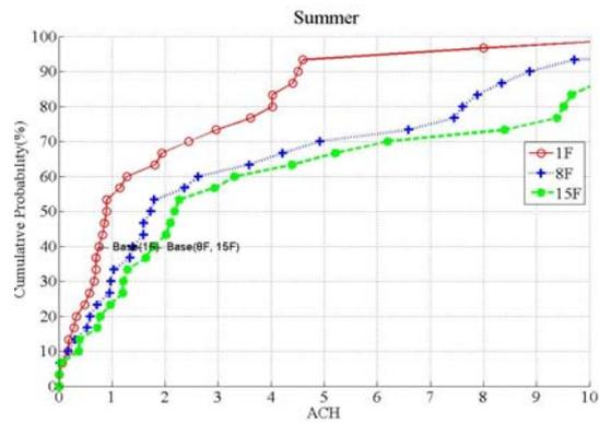
Figure 5 Cumulative probability of natural airflow rates
