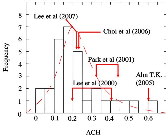
Figure 3 Comparison between the simulated and measured infiltration rates
