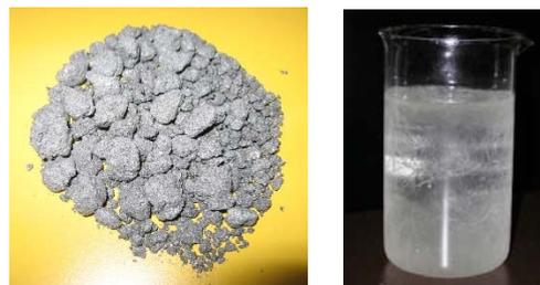
Figure 7 Sodium acetate with graphite (left) and paraffin RT27 (right)
