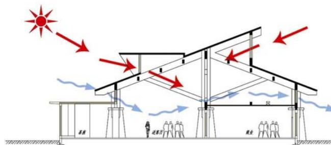
Figure 6. Wind and daylighting routes through pitched roof and openings
