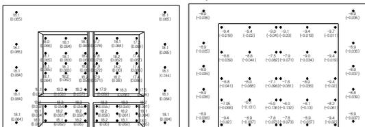
Figure 10 Surface temp. and TDR<sub>i</sub>, TDR<sub>o</sub> (Simulation)
