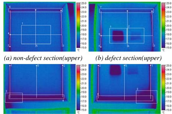
Figure 11 Infra-red thermal imaging data
