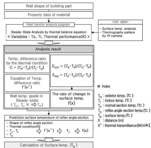
Figure 2 Process for predicting model surface temperature of reflex angle wall sections
