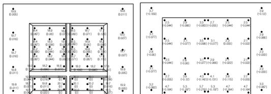
Figure 12 Surface temp. and  $TDR_i$ ,  $TDR_o$ (T-type sensor)
