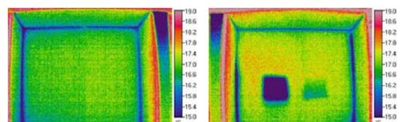
Figure 7 Infra-red thermal imaging data before emissivity adjustment
