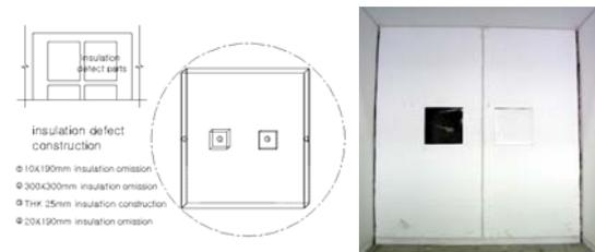
Figure 5 Insulation defects in mock-up structure
