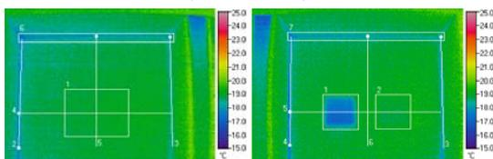
(a) non-defect section(upper) (b) defect section(upper)
