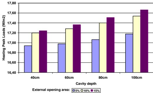
Fig 9 Heating Peak Loads for 1 floor Corridor Façades
