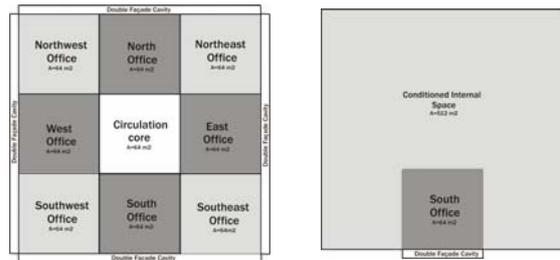
Fig. 2. Building organization and solar orientation for the complete model(left) and for the simplified model (right)
