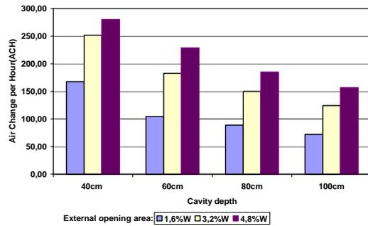
Fig 23 Airflow rates at 6<sup>th</sup> floor cavity for the multistory façades
