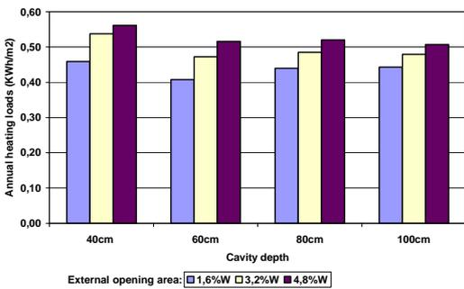
Fig 20 Annual Heating Loads for Multistory wide openings façade typology
