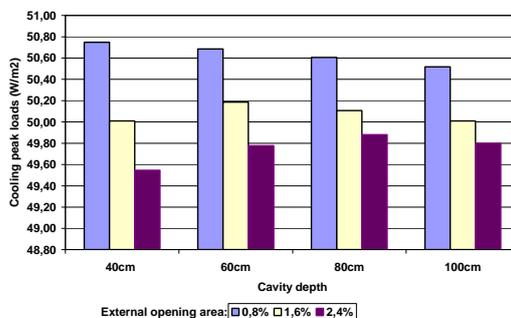
Fig 13 Cooling Peak Loads for Multistory Façades
