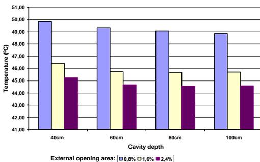
Fig 16 Maximum temperature at 6<sup>th</sup> floor cavity for multistory façades
