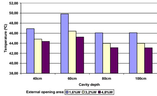
Fig 22 Maximum temperature at 6<sup>th</sup> floor cavity for the multistory façades
