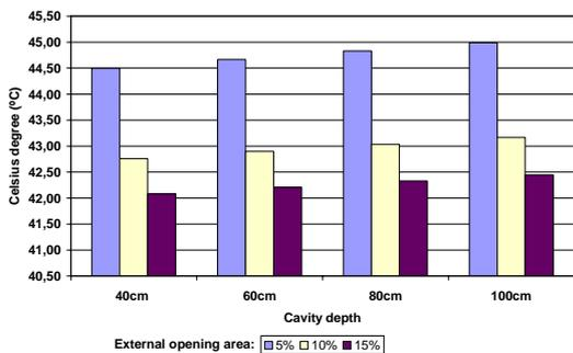
Fig 11 Maximum temperature for 1 floor Corridor façades
