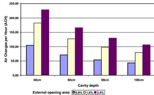
Fig 17 Airflow rates at 6<sup>th</sup> floor cavity for the multistory façades
