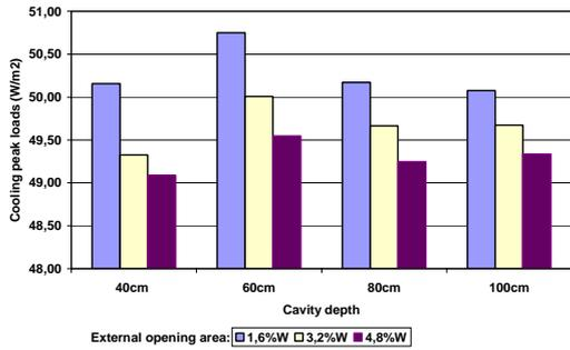
Fig 19 Cooling Peak Loads for Multistory wide openings façade typology
