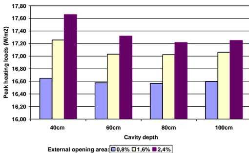
Fig 15 Heating peak Loads for Multistory Façades
