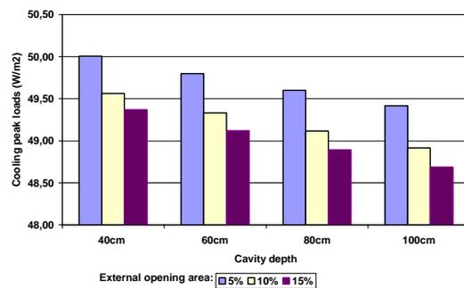
Fig 7 Cooling Peak Loads for 1 floor Corridor Façades
