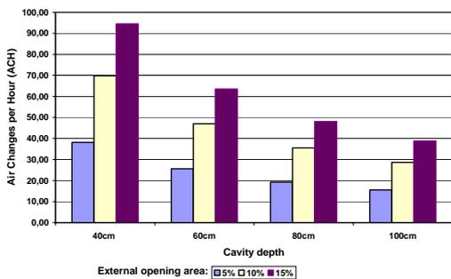
Fig 10 Air changes per hour at the 6<sup>th</sup> floor of the 1 floor Corridor façades
