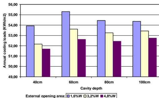
Fig 18 Annual Cooling Loads for Multistory wide openings façade typology
