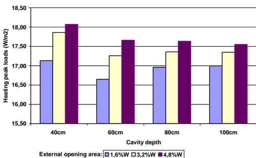
Fig 21 Heating Peak Loads for Multistory wide openings façade typology
