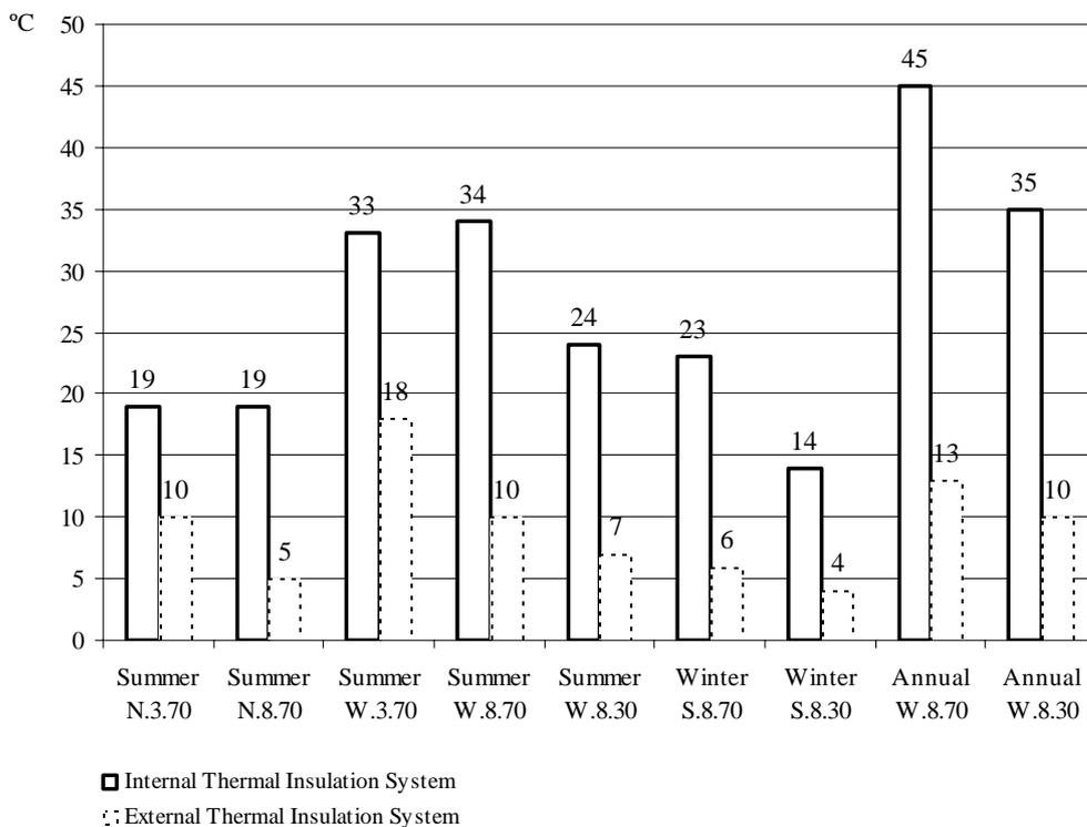
Figure 2 Maximum temperature amplitude across the external masonry wall with external and internal thermal insulation systems, under severe summer, winter and annual Portuguese climate conditions (city of Porto) (each column represent a different combination of wall orientation (N, S, or W), thickness of thermal insulation material (3 or 8 cm) and solar radiation absorption coefficient (0.70 or 0.30).
