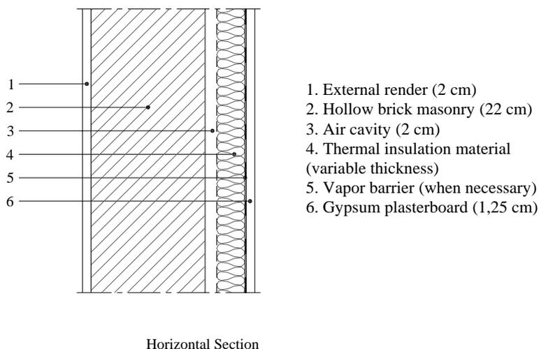
Figure 1 Scheme of the studied internal thermal insulation system.
