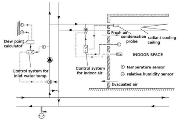
Figure 1 Central control of water temperature and local detection of the condensation
