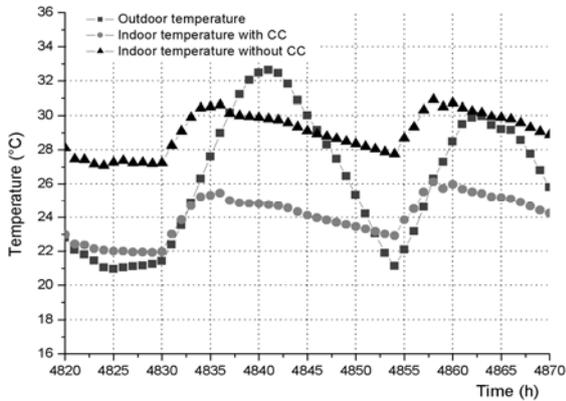
Figure 4 Office room air temperatures for two days simulation with/without the cooling ceiling (CC)
