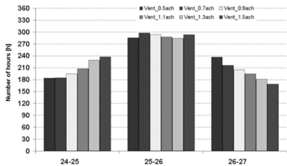
Figure 7 Air temperatures distribution when using the CC and for different ventilation rates
