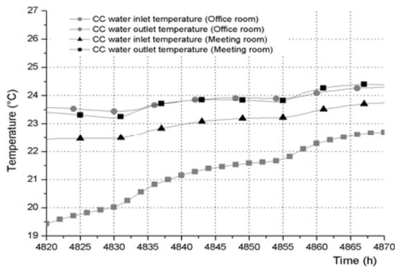
Figure 5 Inlet/outlet water temperatures of the CC for the two indoor spaces
