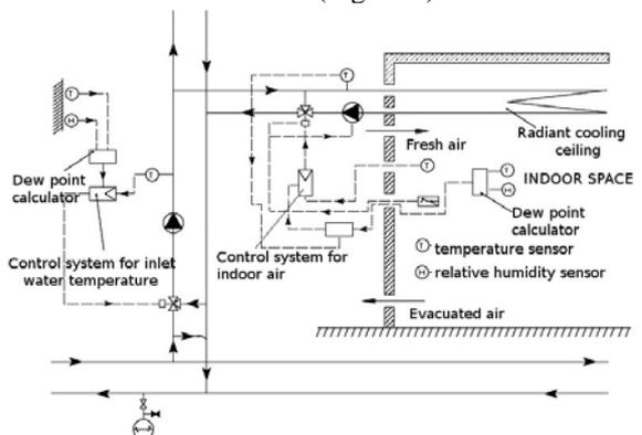
Figure 2 Central and local control of water temperature with zone surveillance
