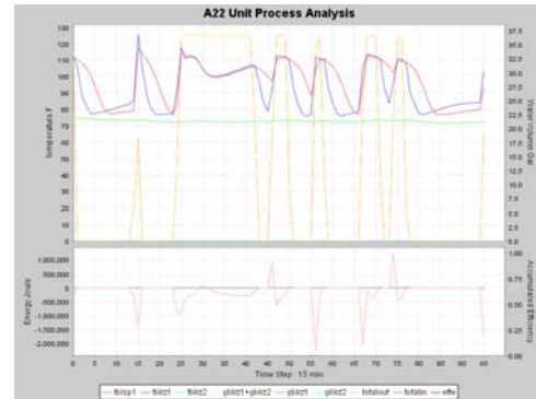
Figure 16. Composite view: efficiency table and A22 "space heating boiler" process unit energy conversion efficiency graph (date: 2004-302)
