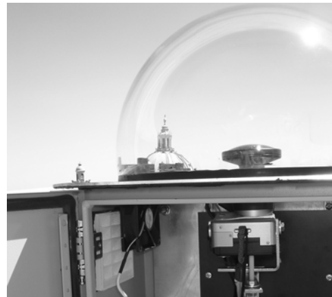
Figure 1 Digital camera with fisheye lens
