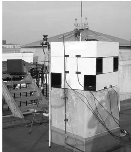
Figure 2 Sky monitoring device, digital camera with fisheye converter and illuminance meter
