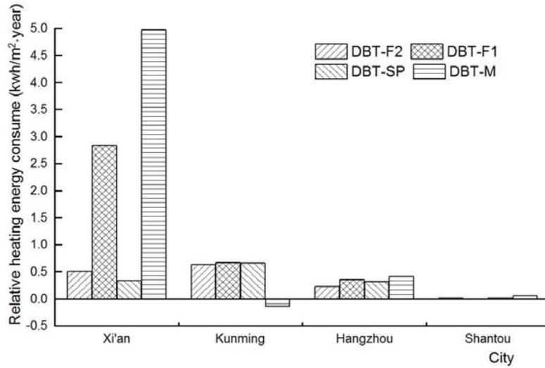
Figure 1. Relative heating energy consumption in the four cities with different hourly DBT data
