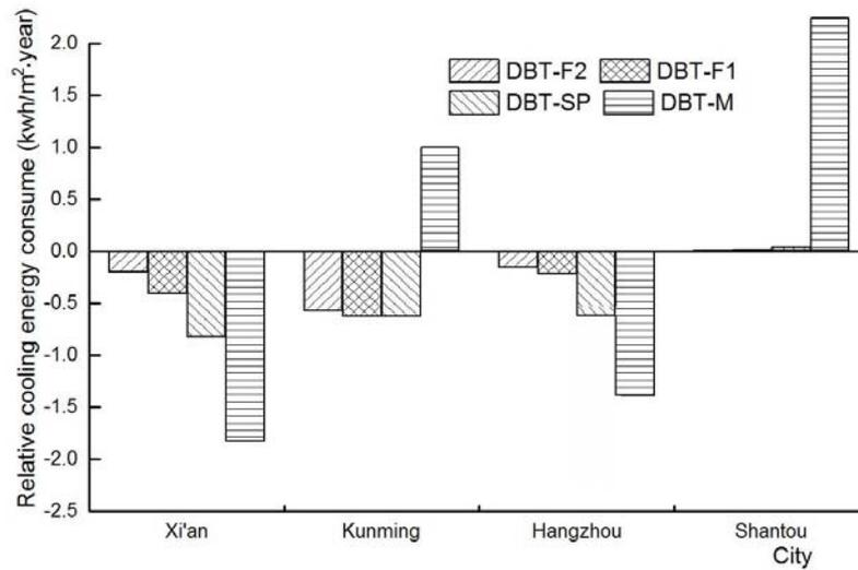
Figure 2 Relative cooling energy consumption in the four cities with different hourly DBT data
