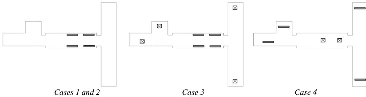
Figure 4 Cases according to the location of air in/outlet
