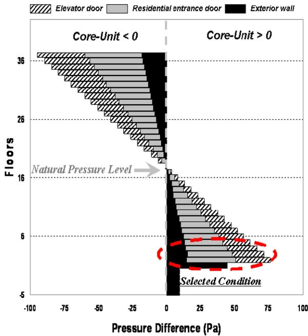
Figure 2 Pressure difference and airflow direction
