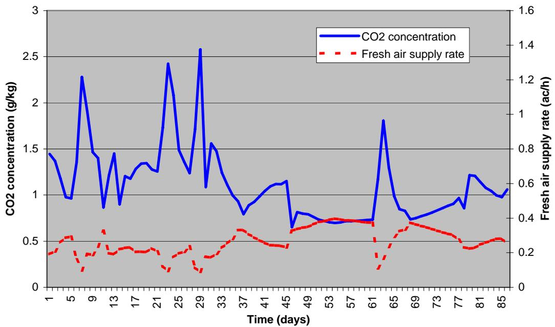
Figure 4. CO2 concentration and fresh air supply rate vs time.
