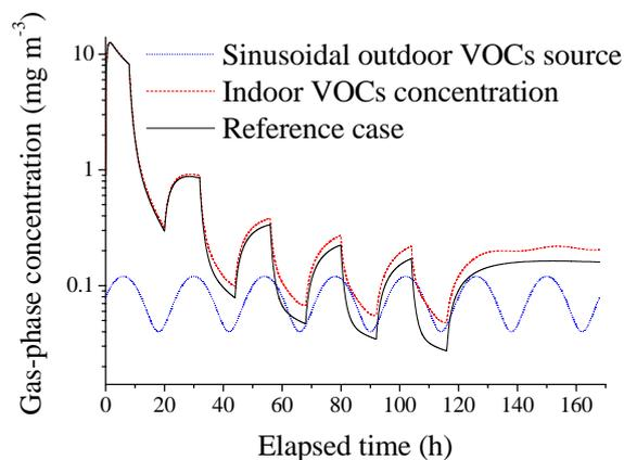
*Figure 5 Impact of outdoor VOCs sources on indoor VOCs concentration*
