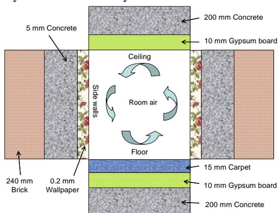
Figure 1 Structures of sidewalls, ceiling and floor
