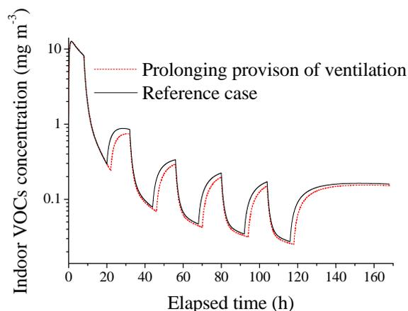
*Figure 4 Impact of prolonging provision of ventilation on indoor VOCs concentration*
