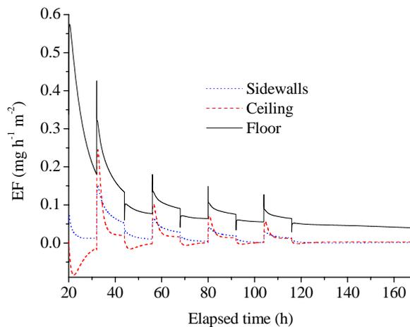
*Figure 2 Behaviors of emission factors from different building components under the Reference case*
