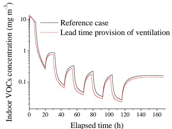
*Figure 3 Impact of lead-time provision of ventilation on indoor VOCs concentration*
