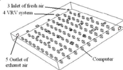
Figure 3 the 3D Schematic for Restructured VRV System
