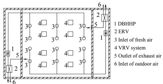
Figure 2 the Schematic for Restructured VRV System
