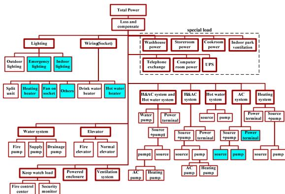
Figure 4 EC data structure of building A
