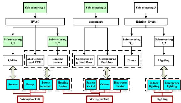
Figure 8 Relation between sub-metering and EC structure of building A
