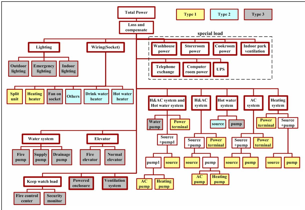
Figure 1 Unified tree structure of energy consumption data.
