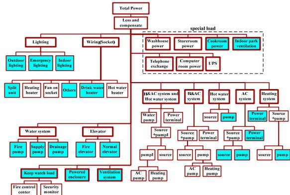
Figure 5 EC data structure of building B
