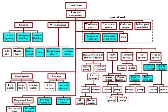
Figure 7 EC data structure of building D
