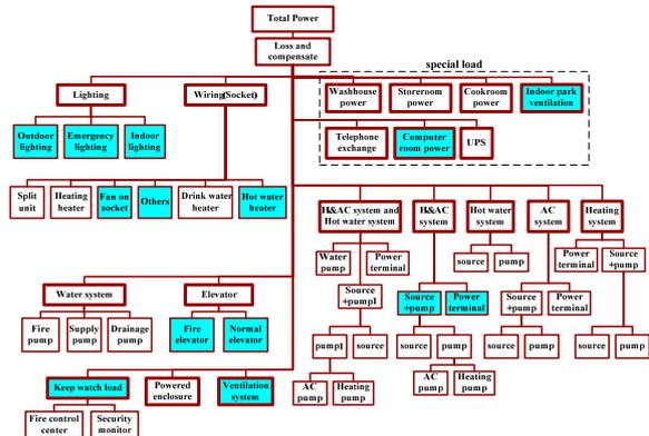
Figure 6 EC data structure of building C
