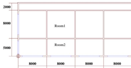
Figure 13 Layout plan of the Case Study Building (Unit: mm)
