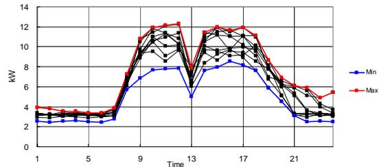
Figure 1 A Japanese office's 8 days measured equipment electricity consumption in 2004
