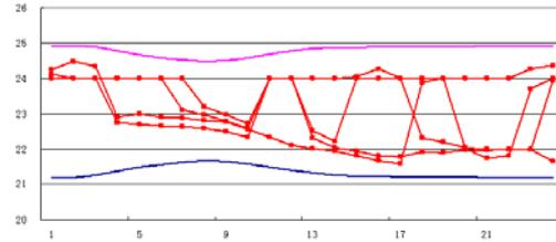
Figure 12 One day's hourly indoor temperatures of Case 2
