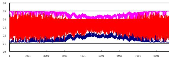
Figure 11 Full year hourly indoor temperatures of Case 2
