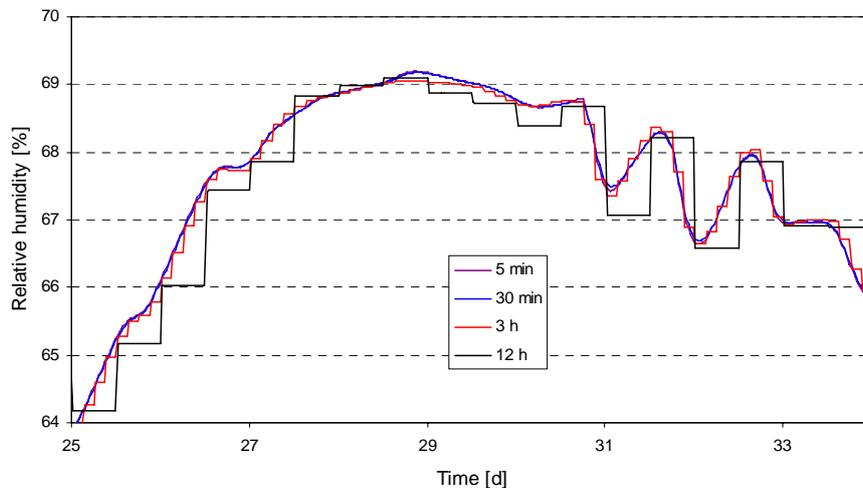
Fig. 6 Stepwise change of zone RH for larger exchange intervals
