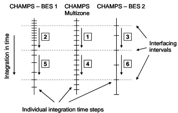
Fig. 4 Integration and interfacing principle
