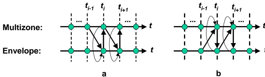
Fig. 3 Coupling schemes in time integration ( $t_i$  = current integration time point)
