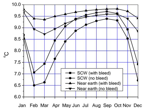
Figure 5 Mean well water temperatures and local rock temperatures for the 4 well cluster ('near earth' represents the earth temperature 1m from well centre)
