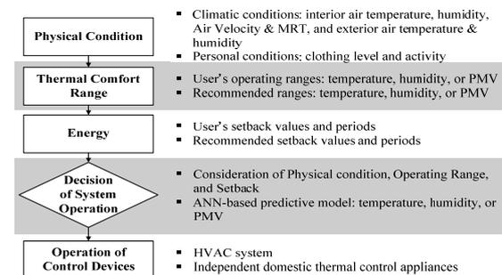
Figure 1 Framework of the thermal control logic
