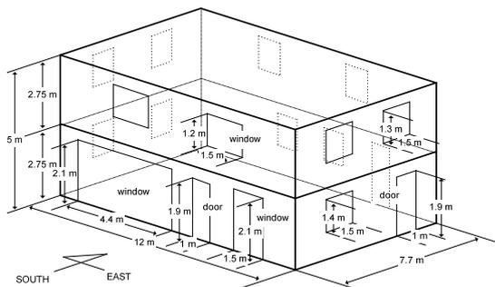
Figure 4 View of a target building
