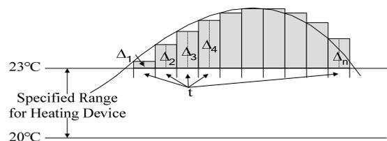
Figure 6 Magnitude of Overshoot of Air Temperature
