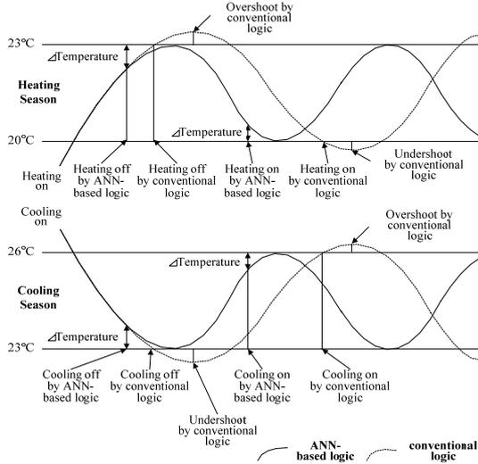
Figure 2 Comparison of air temperature profile between a conventional and a predictive logic
