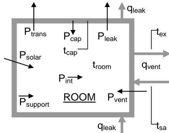
*Figure 3 Power balance used in the simulation tool for the building. The air handling unit is not shown. Quantities are given in the text.*
