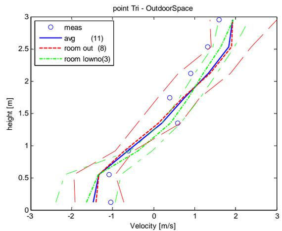
Figure 3 Difference in modelling a high outdoor space compared to modelling without such a space or a low outdoor space (for point J and  $\Delta$  respectively).
