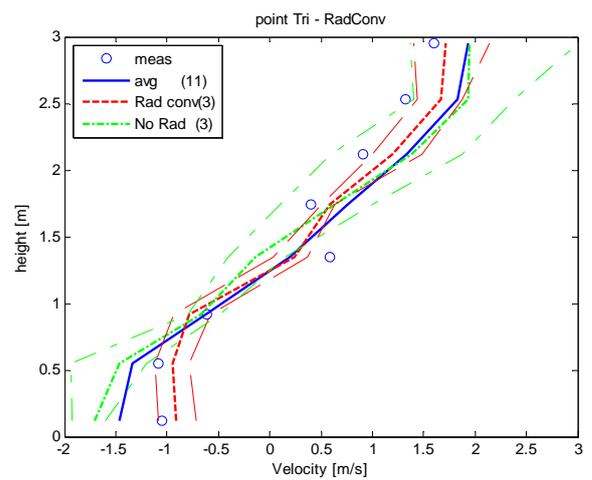
Figure 6 Difference in including radiant heat transfer; radiation taken into account in the convective heat source compared to neglecting the radiant part completely.
