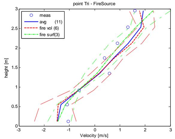
Figure 4 Difference in modelling of a fire; volumetric heat source approach compared to heat release at a surface.
