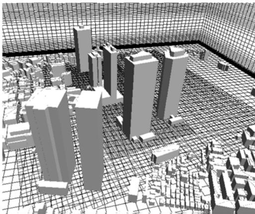
Figure 2 Part of geometry and computational grid for CFD study of pedestrian-level wind conditions in the Shinjuku Sub-central area in Tokyo, Japan (Yoshie et al., 2007).
