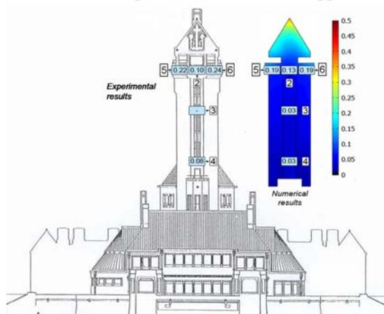
Figure 5 Comparison of measured and simulated catch ratio on the south-west facade of the tower of the monumental building St. Hubertus in the Netherlands (Briggen et al., 2009).
