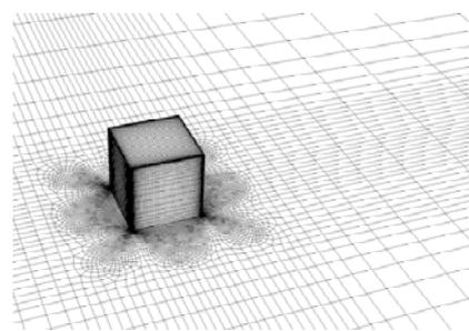
Figure 6 High-resolution grid for CFD simulation of convective heat transfer coefficients around an isolated cubic building model, with first grid cell point at 160  $\mu$ m from the facade (Blocken et al., 2009).
