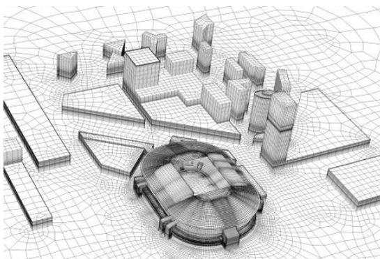
Figure 3 Part of geometry and computational grid for CFD study of pedestrian-level wind conditions around the Amsterdam “ArenA” football stadium in the Netherlands (Blocken and Persoon, 2009).
