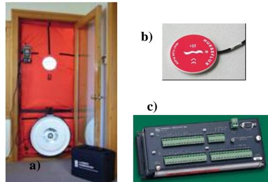
Figure 4 “in-situ” measurement equipment, a) blower-door, b) heat flux meter; c) data-logger
