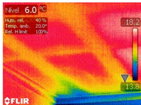
Figure 6 infrared picture – identification of roof structure (CS1)
