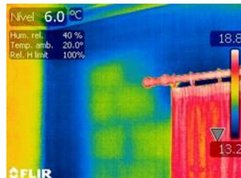
Figure 5 infrared picture – identification of thermal bridges (CS1)
