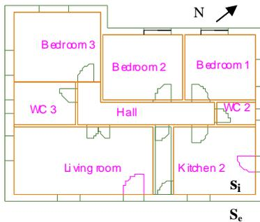
Figure 3 Quinta do Canelas floor plans;  $S_i$ ,  $S_e$  – positioning of interior and exterior heat flux sensor and thermocouples, respectively
