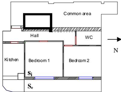
Figure 2 Viseu floor plans;  $S_i$ ,  $S_e$  – positioning of interior and exterior heat flux sensor and thermocouples, respectively
