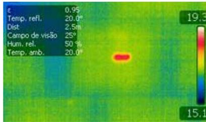
Figure 7 infrared picture – positioning the heat flux meter (CS1)
