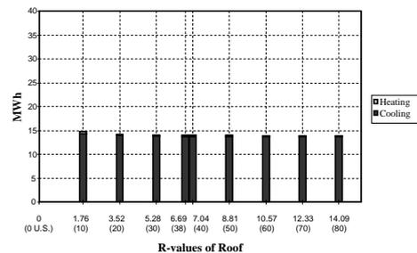
Figure 16 Heating and Cooling Energy Consumption for Various Roof R-values (Miami, Florida)
