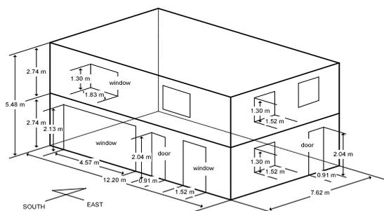
Figure 1 South-East Exteriors of the Test Building
