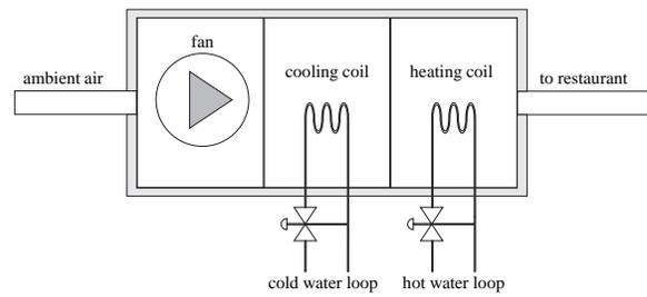
Figure 3: Schematic of air handling unit. The main elements are a fan, and cooling and heating coils.
