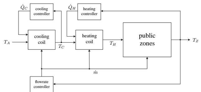
Figure 4: Block diagram of restaurant control system. Variables are defined in table 1.
