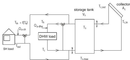
Figure 7 Solar combisystem model layout
