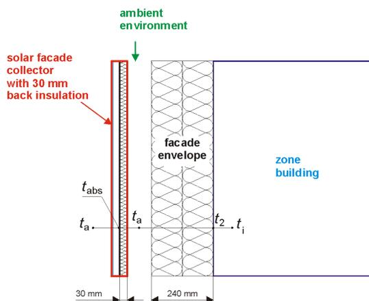
Figure 3 Indirect integration of solar collector considered as a separate installation
