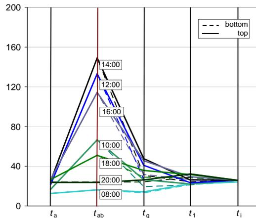
Figure 6 Temperature profiles in façade with indirectly integrated atmospheric flat-plate collector during summer day
