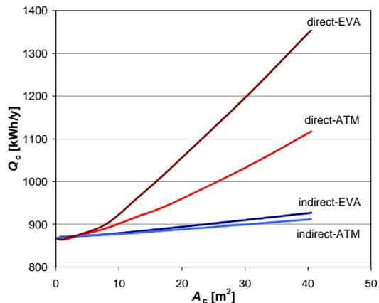
Figure 10 Space cooling demand increase induced by solar collector integration into facade
