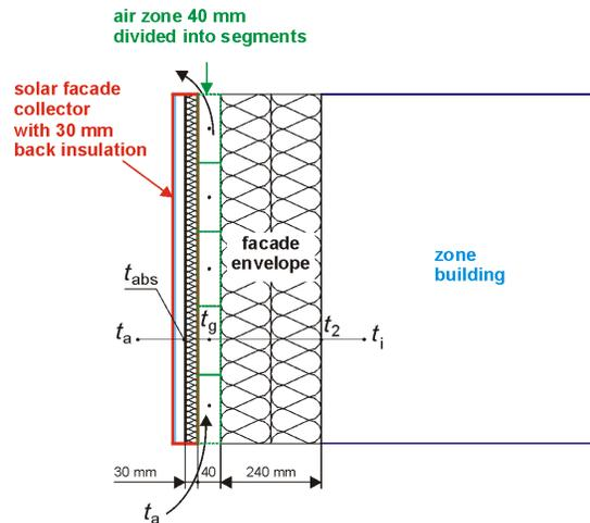
Figure 5 Indirect integration with ventilated air gap.
