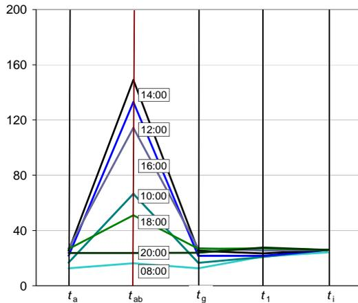
Figure 4 Temperature profiles in façade with indirectly integrated (no TRnflow) atmospheric flat-plate collector during summer day
