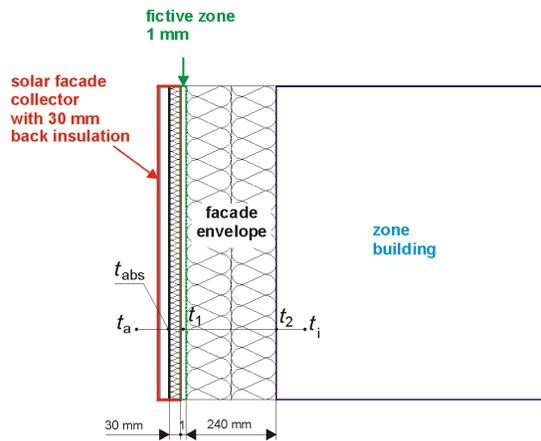
Figure 1 Direct integration of solar collector into the building envelope without air gap
