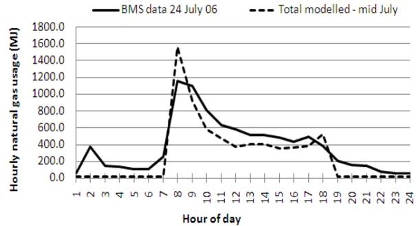
Figure 12 Building Two – Hourly gas data from BMS compared with modelled
