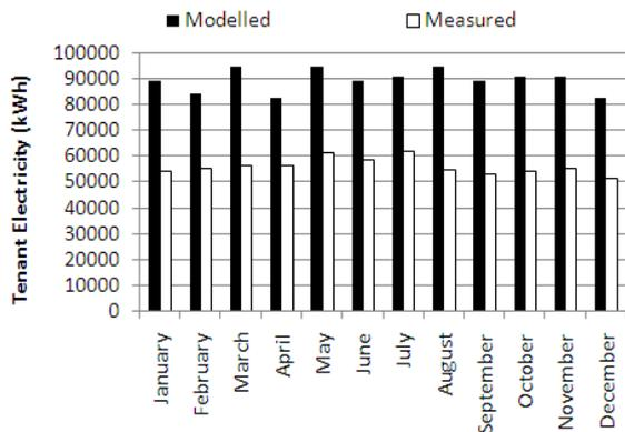
Figure 19 Building Three – Electricity used for tenant light and power
