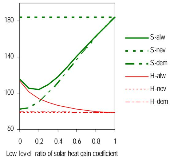
*Figure 2* The ratio between the solar heat gain in the shaded state and the solar heat gain in the non shaded state for the office building.
