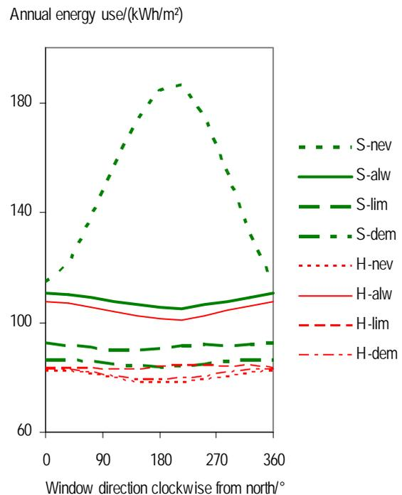
Figure 10 Window normal direction was varied from the default which was 180°, south. 0° and 360° are the same direction, north.
