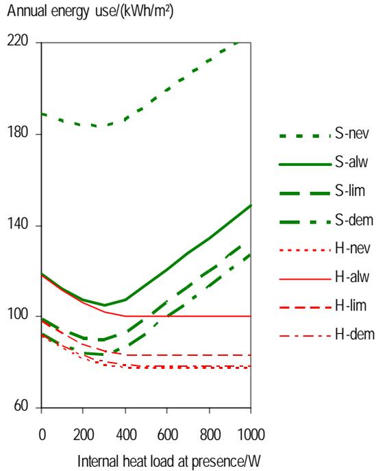
Figure 7 The internal heat load at presence was varied. At absence, it was zero all the time. The default, 340 W, is close to the optimal level regarding the sum of the heating and cooling energy use.
