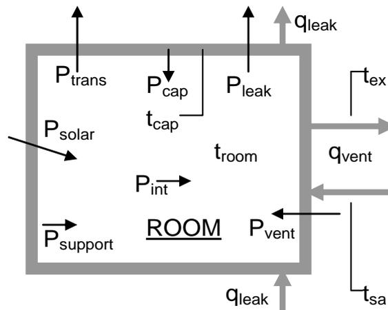
*Figure 1 Power balance used in the simulation tool for the buildings. The air handling unit is not shown. Quantities are given in the text.*
