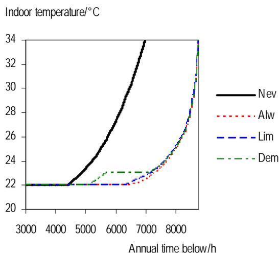
Figure 12 The permanence of indoor temperatures for the apartment for the different solar shading strategies. In the apartment simulation, there was no cooling power available.
