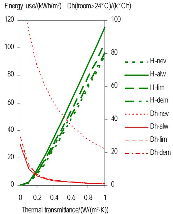
Figure 13 The average thermal transmittance was varied for in the apartment simulation. The right y-axis shows the number of degree hours, Dh over 24°C.
