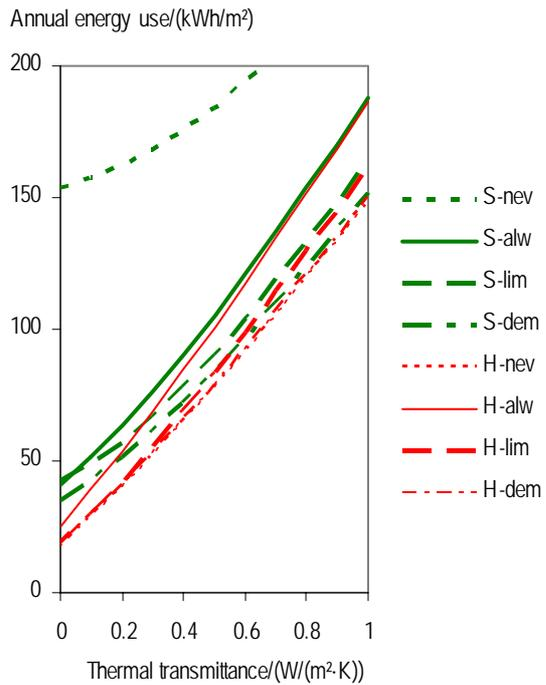
Figure 4 The average thermal transmittance was varied for the office building. At zero, the energy use depends on heating supply air and leakage air.
