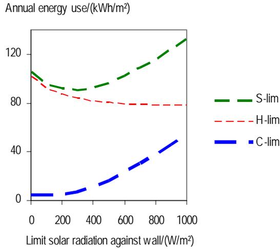
Figure 3 Limit of incoming solar radiation against the wall when the state of the solar shading was changed in the 'Lim' case for the office building. 300 W gives a minimal sum of heating and cooling energy use.
