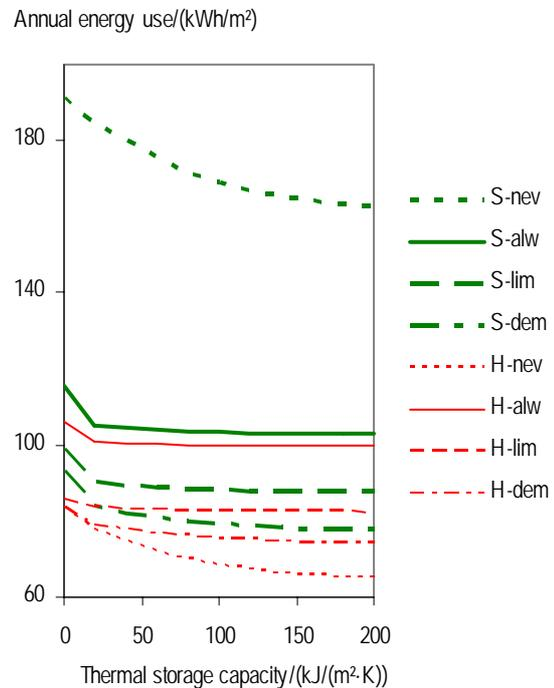
Figure 6 The thermal storage capacity of a m<sup>2</sup> of thermally active indoor material was varied.
