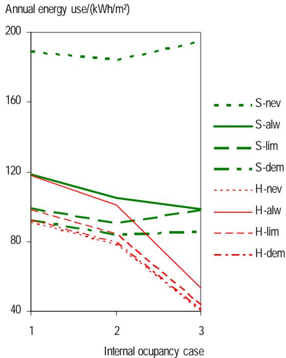
Figure 11 Internal occupancy cases are numbered 1, no occupancy at all, 2, default occupancy, 60% between 08 and 18 4 days a week, and 3, occupancy all the year.
