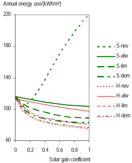
Figure 5 The solar heat gain coefficient of the window was 0.7 in the default case. It was assumed in the model that the solar heat gain coefficient included a possible shading effect from the surrounding.
