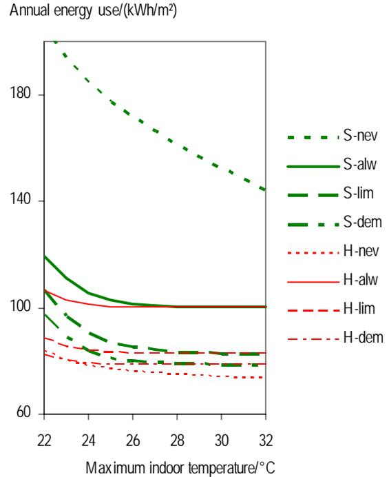
Figure 9 A maximum indoor desired temperature of 22°C is the same as the minimum indoor temperature which disables the heat storage. At approximately 28°C, there was no cooling need.
