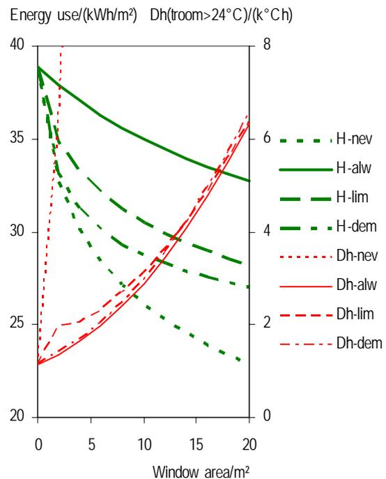
Figure 14 The window area was varied for the apartment. The average thermal transmittance was kept constant.
