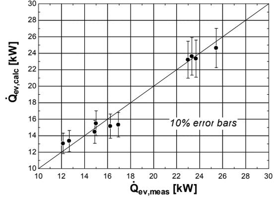
Figure 10 Prediction of the cooling power (chiller model)
