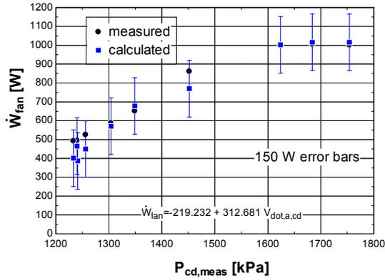
Figure 9 Prediction of the fan electrical consumption (chiller model)
