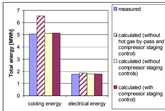
Figure 15 Total cooling and electrical energies over the entire simulation period
