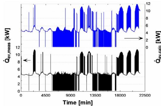
Figure 14 Time evolution of the chiller measured and predicted cooling power
