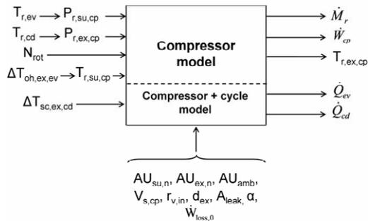
Figure 4 Information diagram of the compressor model
