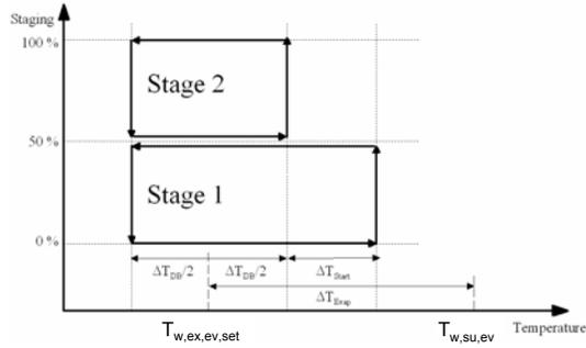
Figure 12 Chiller control scheme
