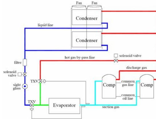
Figure 3 Air-cooled chiller refrigerant circuit
