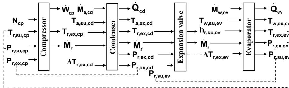
Figure 1 Schematic representation of the chiller model
