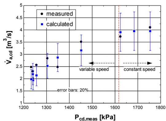
Figure 8 Prediction of the condenser air flow rate (chiller model)
