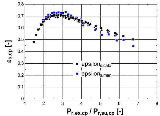
Figure 6 Prediction of the compressor isentropic effectiveness (compressor model)
