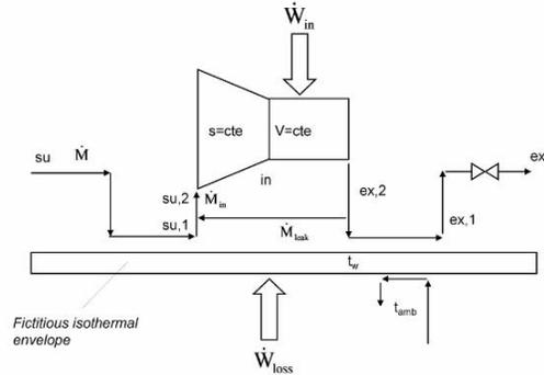
Figure 2 Schematic representation of the scroll compressor model
