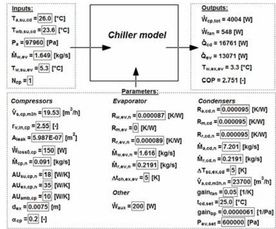
Figure 11 Information diagram of the chiller model
