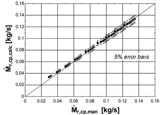
Figure 5 Prediction of the displaced refrigerant mass flow rate (compressor model)
