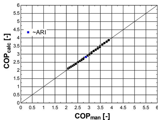
Figure 7 Prediction of the chiller COP (chiller model)
