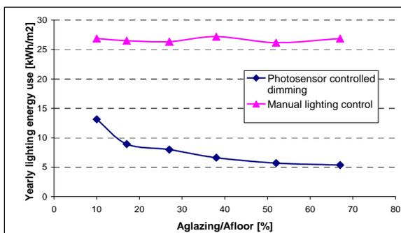
Figure 7 Yearly lighting energy use of manual and dimming light control systems for user type 1, automated blinds, as a function of glazing-to-floor ratio
