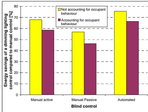
Figure 3 Energy savings of daylight dimming compared to manual control for different blind control systems, with or without accounting for occupant behaviour
