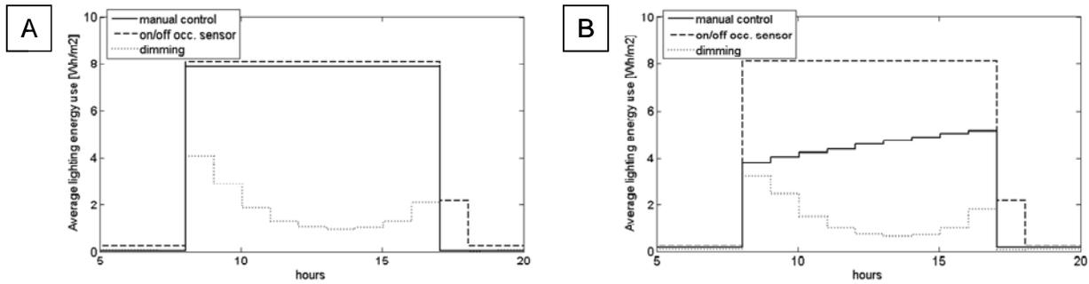
Figure 13 Average daily profile of lighting energy use for different control types (A – user type 2, automated blinds; B - user type 1, automated blinds)
