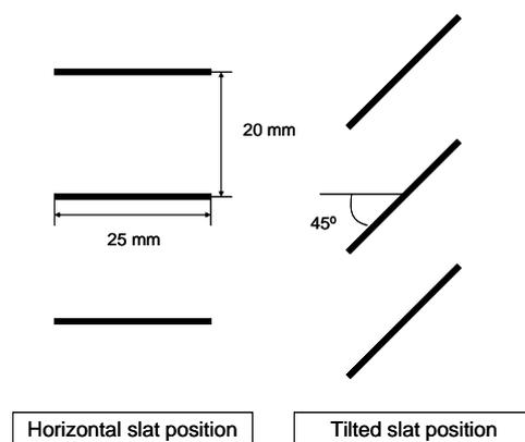
Figure 2 Internal venetian blind geometry
