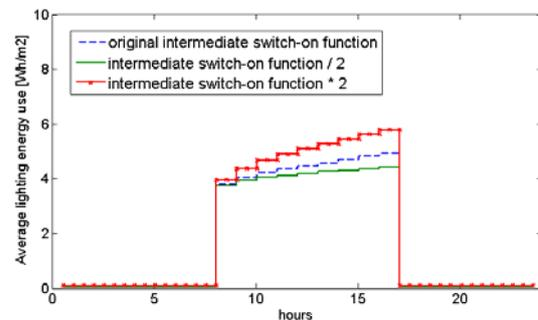
Figure 5 Average daily profile of lighting energy use for user type 1, automated blind control and manual lighting control. Sensitivity on intermediate switch-on probability
