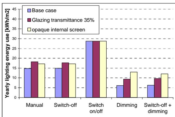
Figure 6 Comparison of the lighting energy use for user type 1, automated blinds for different glazing visual transmittance and screen visual transmittance
