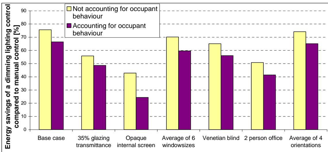
Figure 11 Overview of parameter analysis on the energy savings potential of daylight dimming lighting control compared to manual control, with or without accounting for occupant behaviour
