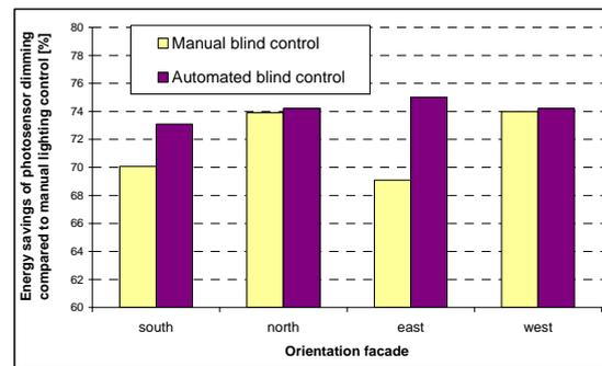
Figure 8 Energy savings of daylight dimming compared to manual control for different orientations and different blind control systems
