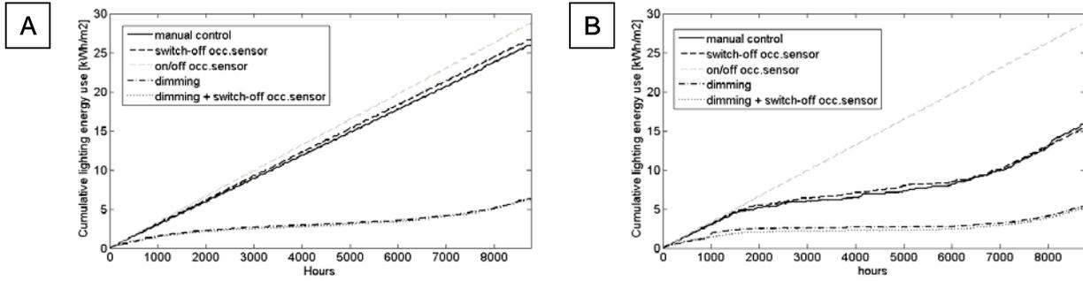
Figure 12 Plots of cumulative lighting energy use for different control types and user types of the base case (A – user type 2, automated blinds; B - user type 1, automated blinds)
